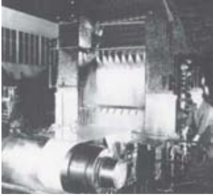
STEEL: Steel sheets are cooled with blades of water from Rex Flat Spray Nozzles.
